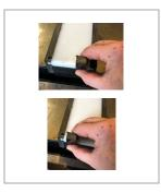
When the blank doesn't just pop right out, you'll want to remove one or both gates. To do this, invert the mold on the bench with one gate hanging over the edge. We have tried to provide a small piece of HDPE scrap to us, but a small block of wood works as well. Find the lip of the gate with the block and gently tap it out.
